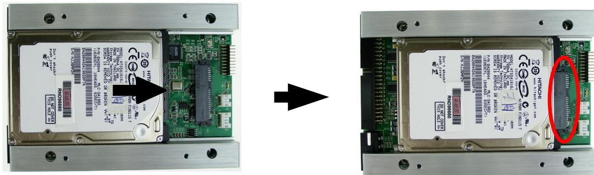
3. Fix the SATA hard drive or SSD to the two sides of SCSIDE2.5U with the enclosed 4 screws.
