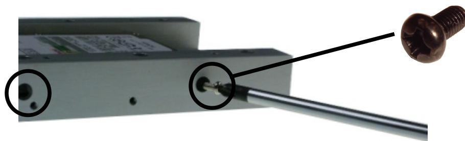
4. Return the upper cover of the SCSIA2.5U bridge and fix it with the 4 screws.
